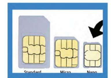
Remove the middle adapter from the adapter pack and place the activated Nano Simin the recess of the adapter.
